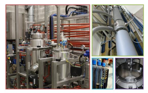
Three pilot plants **Supercritical Fluid Extractors SFE-CO<sub>2</sub>** - 2x 6L/batch + 1 lab-scale equipment
